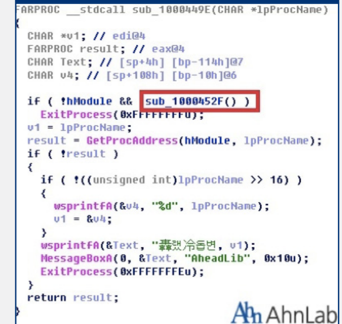
[Fig. 1-8] Malicious code that loads imm32A.dll as sub routine
